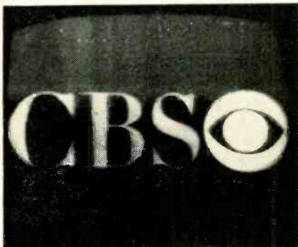
Fig. 7—An excessively dark picture was the symptom; brightness and contrast controls had no effect. See circuit in Fig. 8 for the cause of the problem.
