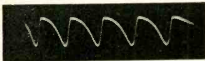
Fig. 6—Different receivers have different methods of obtaining and using vertical sync. This is the sync waveform input to the vertical oscillator in RCA's KCS153 solid-state television chassis.
