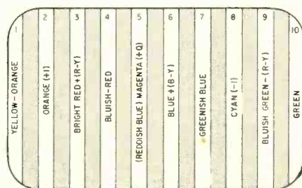
Color-bar generator display on CRT looks like a daisy on the vectorscope display.
