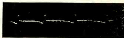
Fig. 4—Waveform at the base of the vertical oscillator transistor shown in Fig. 3-b. The p-p amplitude was low and the signal jittery. Vertical sync in the set was unstable. The coupling capacitor from the sync separator was slightly leaky.
